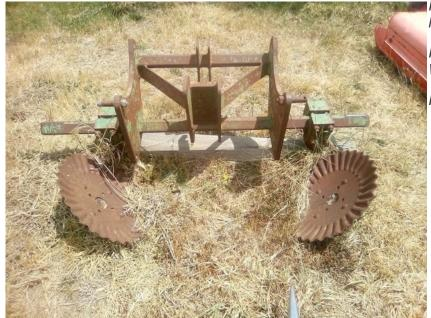
Mounder, attaches to three-point linkage on tractors
