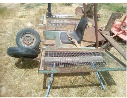
Tractor drawn tree planter, attaches to three-point linkage on tractors
